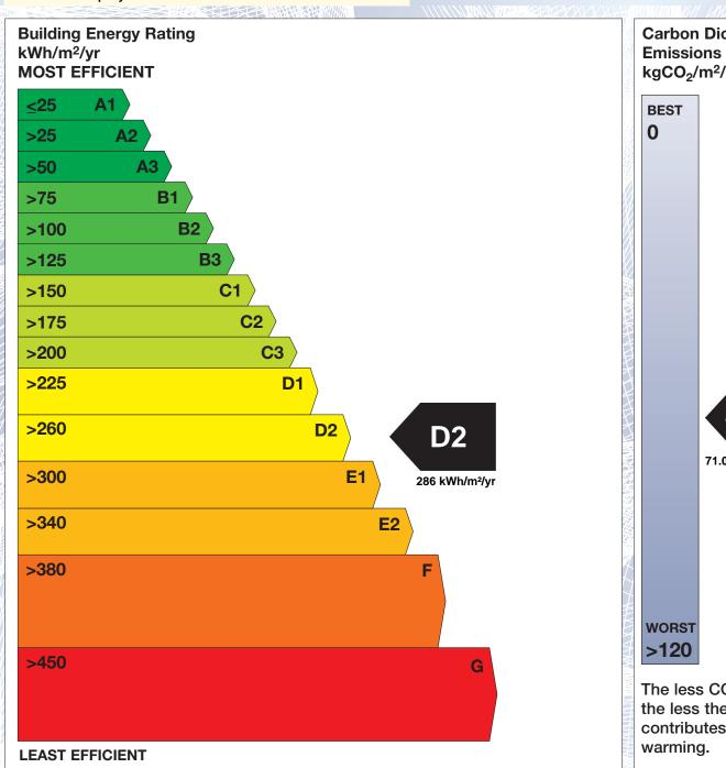
Carbon Dioxide (CO<sub>2</sub>) **Emissions Indicator** kgCO<sub>2</sub>/m<sup>2</sup>/yr Calculated annual CO2 emissions 71.01 kgCO<sub>2</sub>/m<sup>2</sup>/yr The less CO<sub>2</sub> produced, the less the dwelling contributes to global
