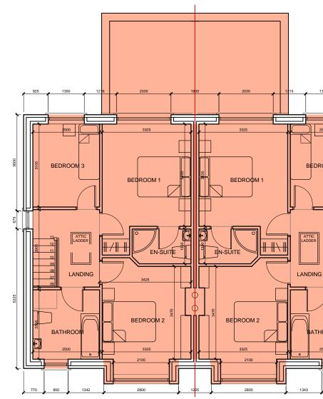
FIRST FLOOR PLAN floor area= 51.5 m<sup>2</sup>
