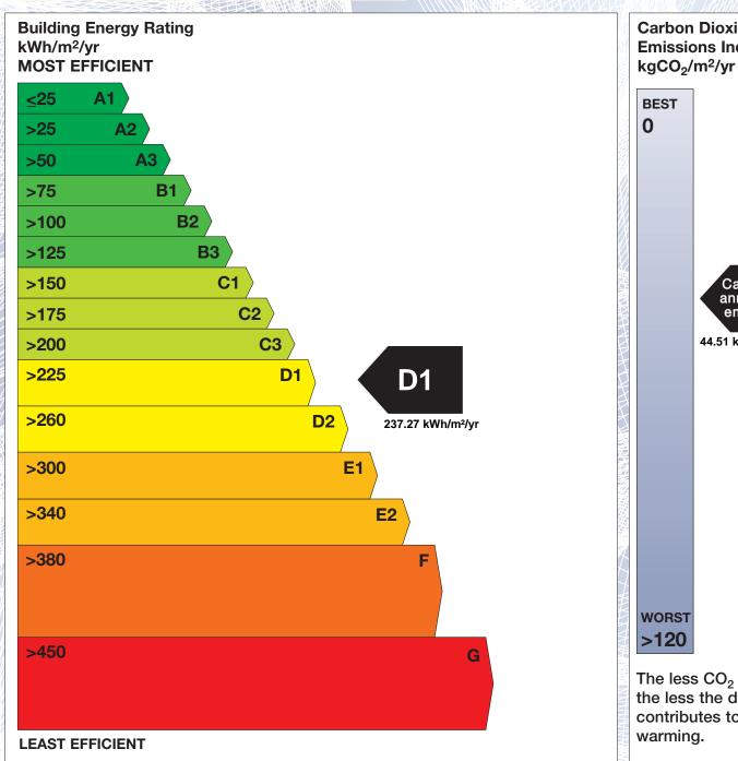
Carbon Dioxide (CO<sub>2</sub>) **Emissions Indicator** Calculated annual CO2 emissions 44.51 kgCO<sub>2</sub>/m<sup>2</sup>/yr The less CO<sub>2</sub> produced, the less the dwelling contributes to global
