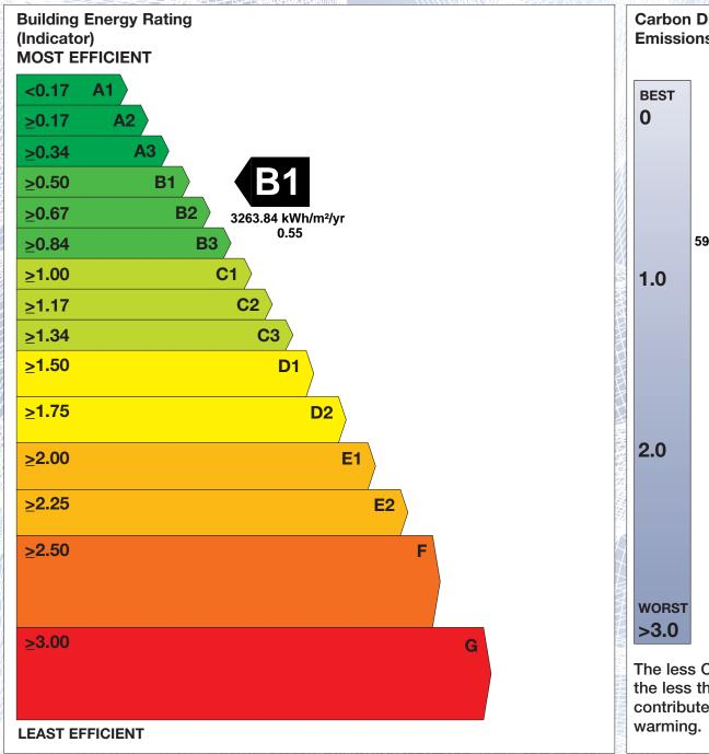
Carbon Dioxide (CO<sub>2</sub>) **Emissions Indicator** Calculated annual CO2 emissions 593.15 kgCO<sub>2</sub> /m<sup>2</sup>/yr 0.54 The less CO<sub>2</sub> produced, the less the building contributes to global
