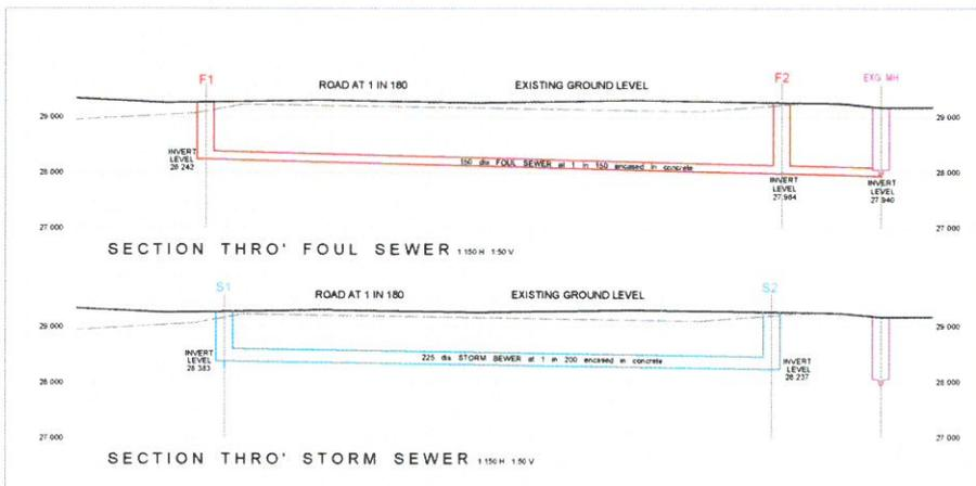
FOUL DRAINS 1000 UPVC AT MINIMUM GRADIENT OF 1 in 60 EXCEPT WHERE SHOWN OTHERWISE. STORM DRAINS ALL 1000 UPVC AT MINIMUM GRADIENTS OF 1 in 80.
