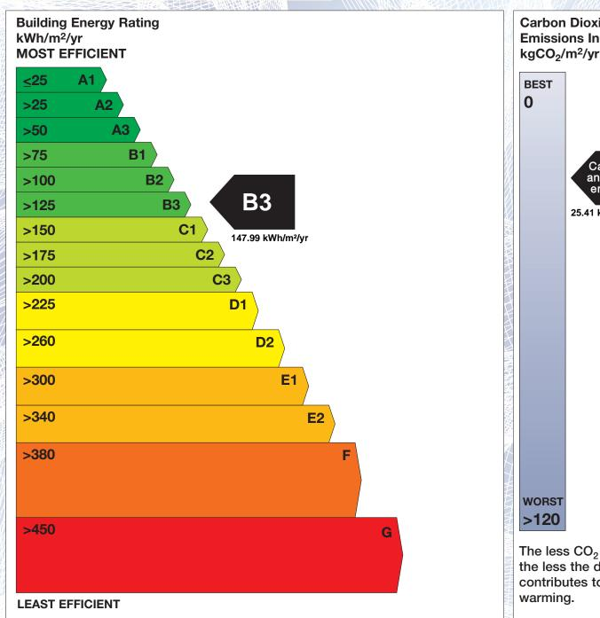
Carbon Dioxide (CO<sub>2</sub>) **Emissions Indicator** kgCO<sub>2</sub>/m<sup>2</sup>/yr Calculated annual CO2 emissions 25.41 kgCO<sub>2</sub>/m<sup>2</sup>/yr The less CO<sub>2</sub> produced, the less the dwelling contributes to global
