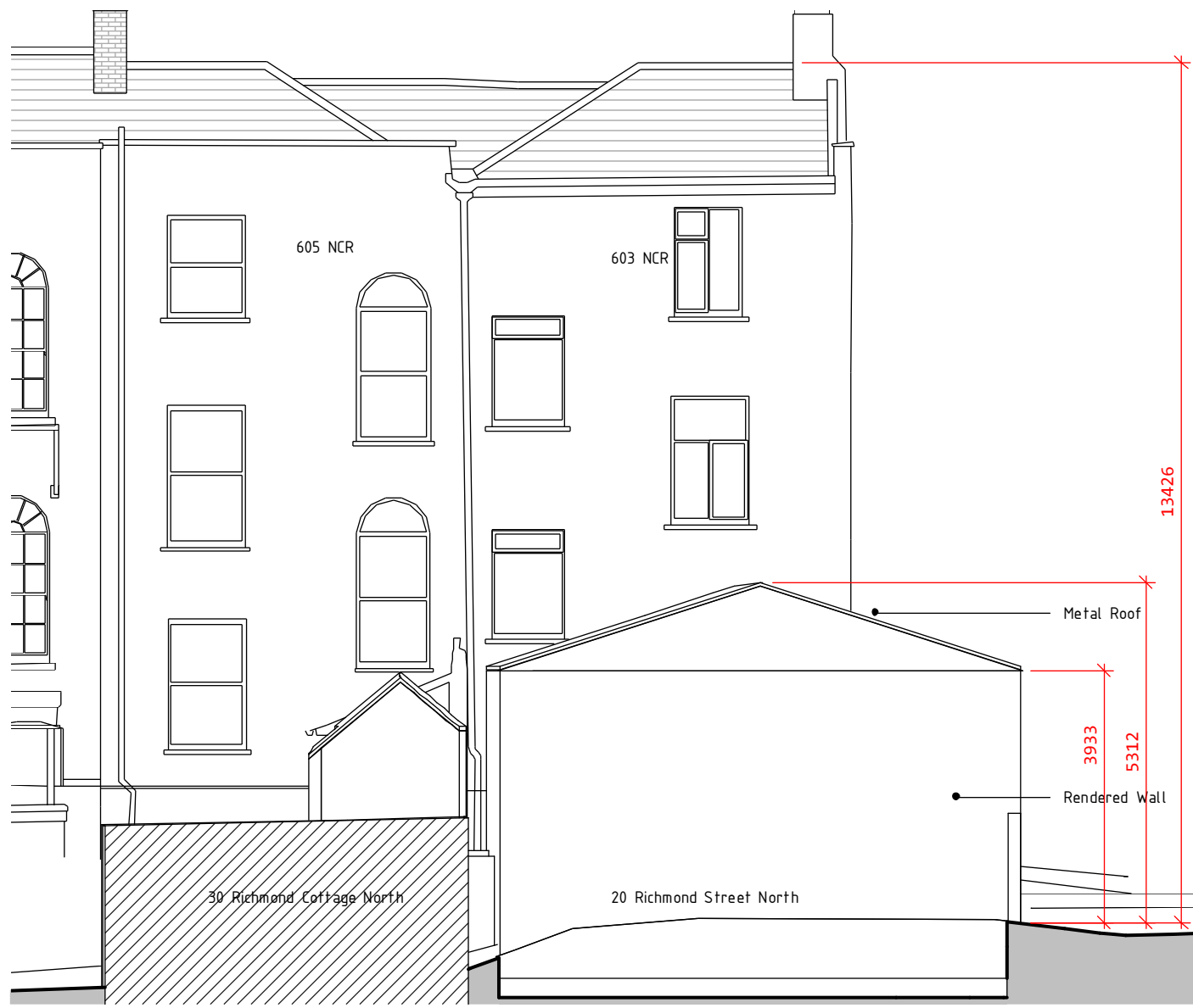
1 Existing North Gable Elevation 106 1 : 100
