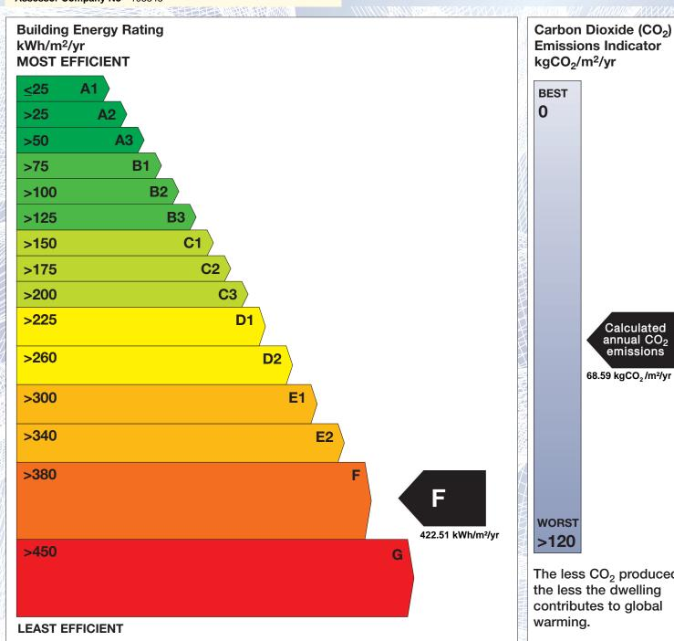
**Emissions Indicator** Calculated annual CO2 emissions 68.59 kgCO<sub>2</sub>/m<sup>2</sup>/yr The less CO<sub>2</sub> produced,
