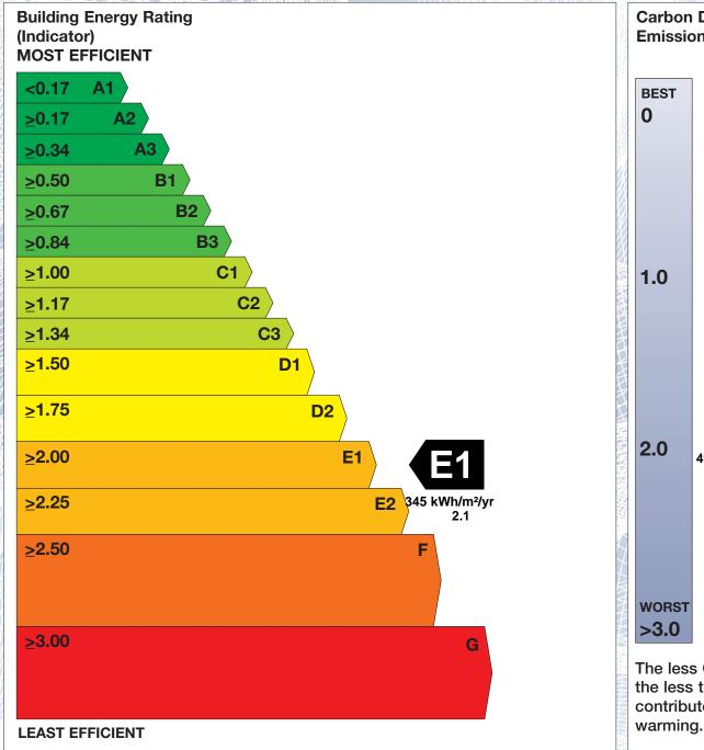
Carbon Dioxide (CO<sub>2</sub>) **Emissions Indicator** Calculated emissions 49.31 kgCO, /m2/yr 1.91 The less CO<sub>2</sub> produced, the less the building contributes to global
