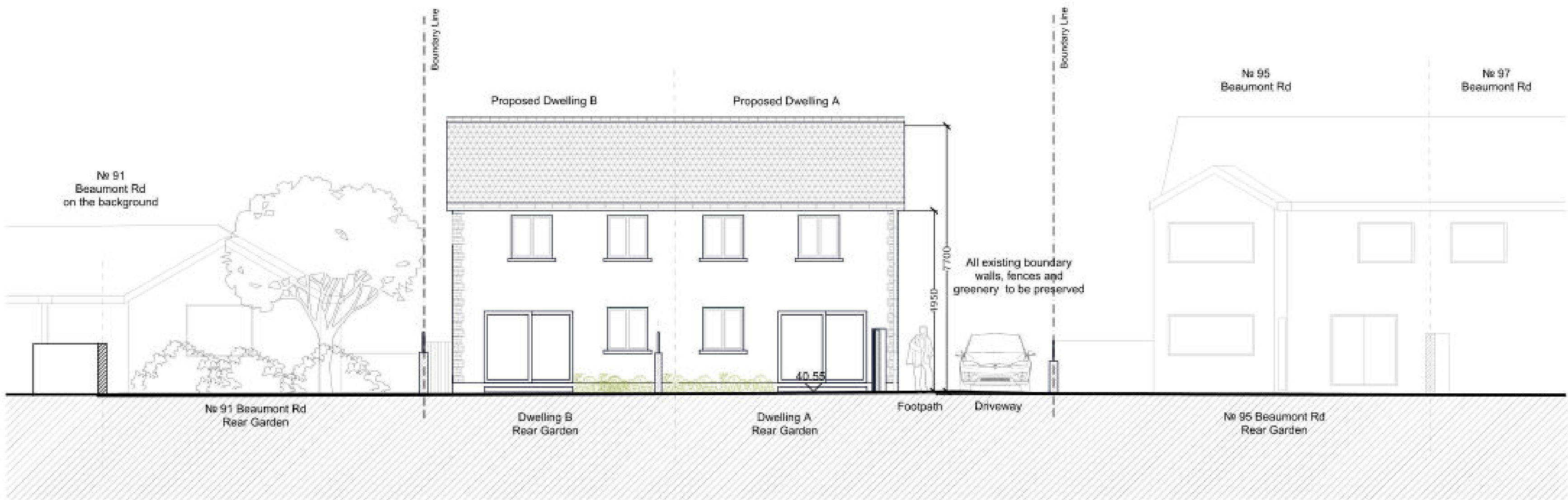
Dwelling A&B Rear Elevation (South-East) Scale 1:100
