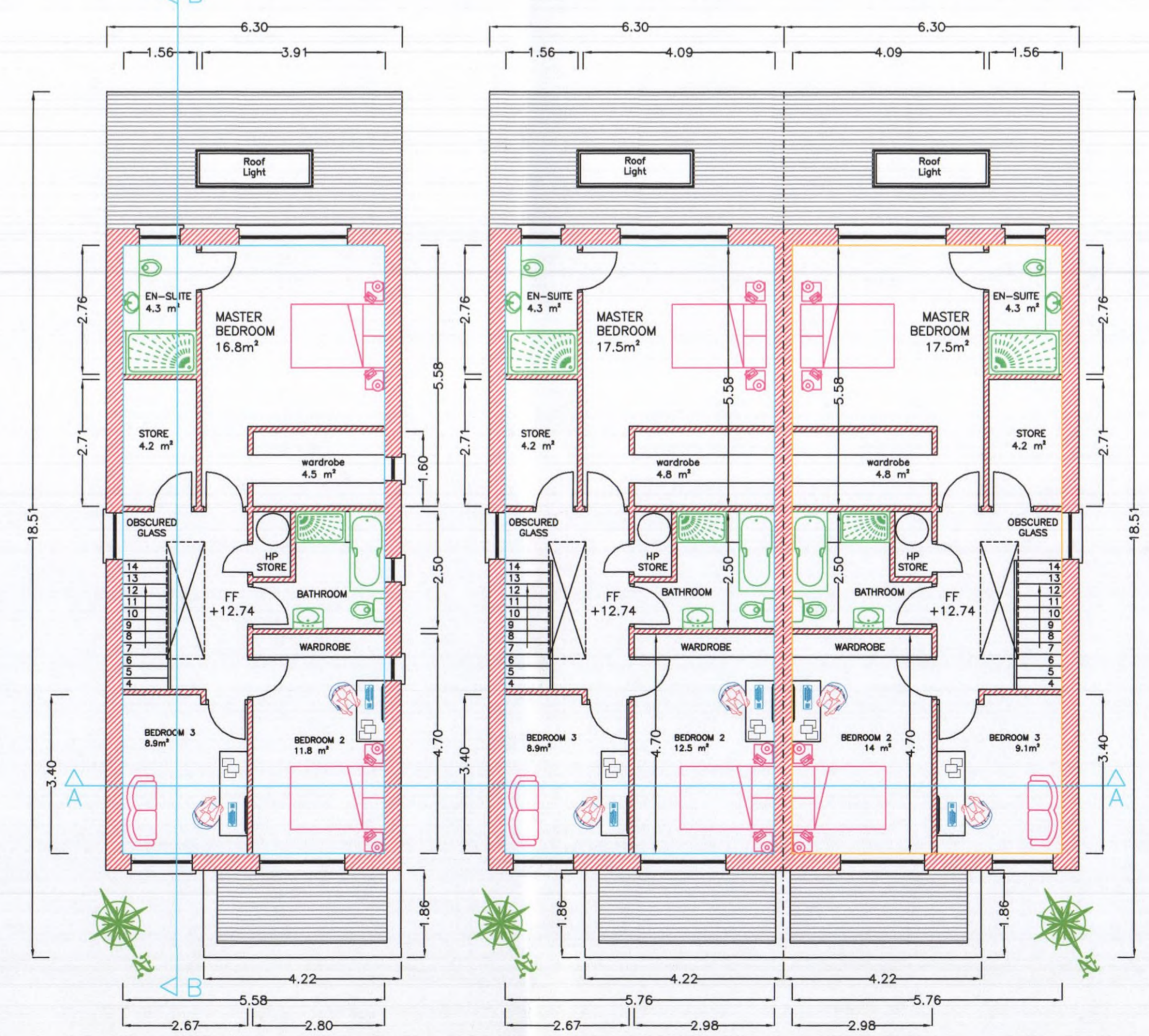
PROPOSED FIRST FLOOR HOUSE 1 Scale 1:100 FIRST FLOOR 72.5 m 2 PROPOSED FIRST FLOOR HOUSE 2 Scale 1:100 FIRST FLOOR 74.9 m 2 PROPOSED FIRST FLOOR HOUSE 3 Scale 1:100 FIRST FLOOR 74.9 m 2
