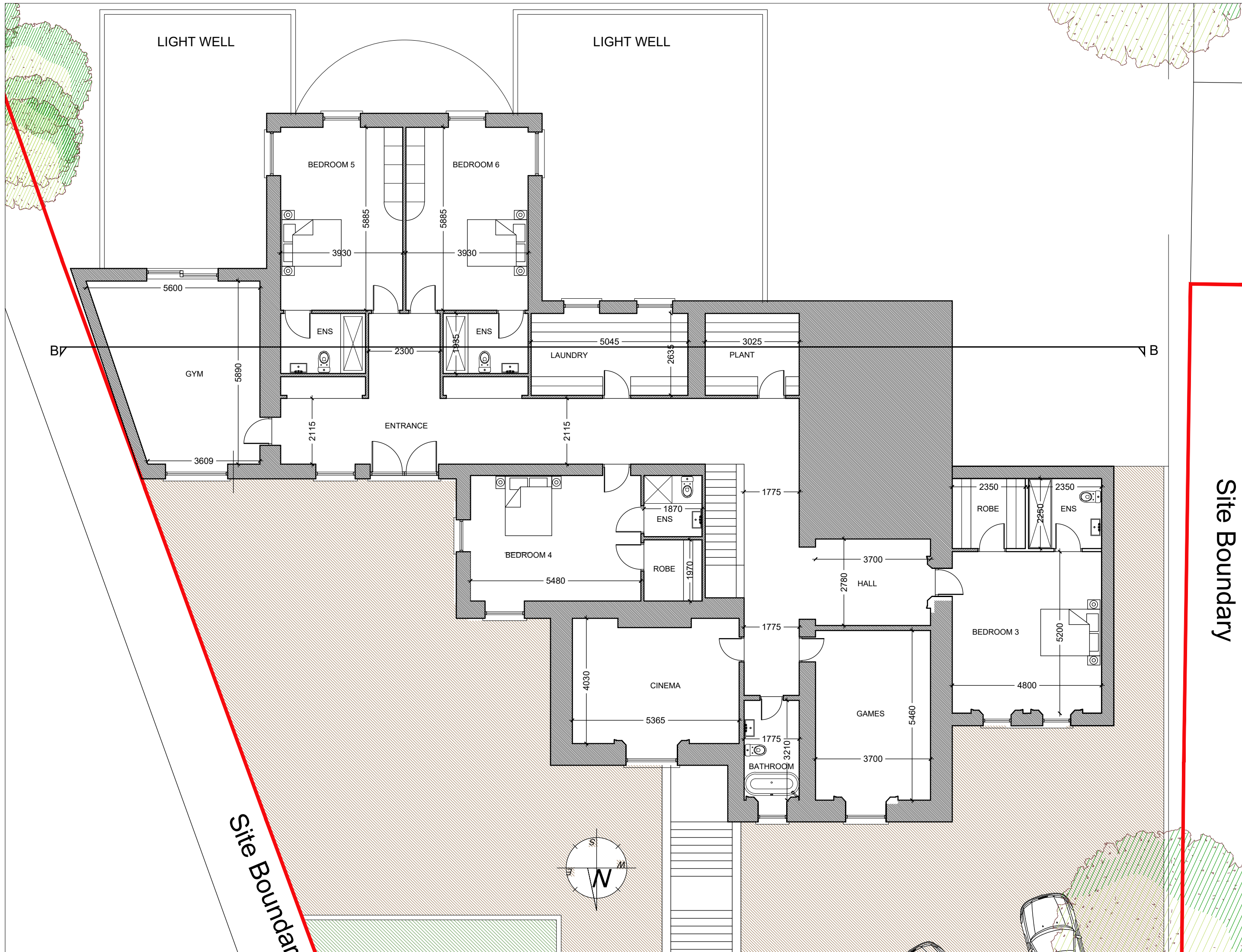
PROPOSED GROUND FLOOR PLAN - 1:100
