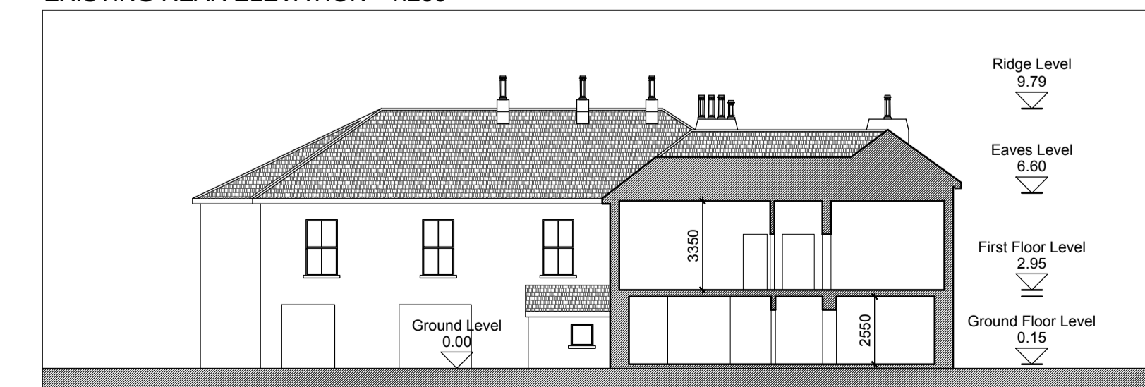
EXISTING SECTION THROUGH A-A - 1:200
