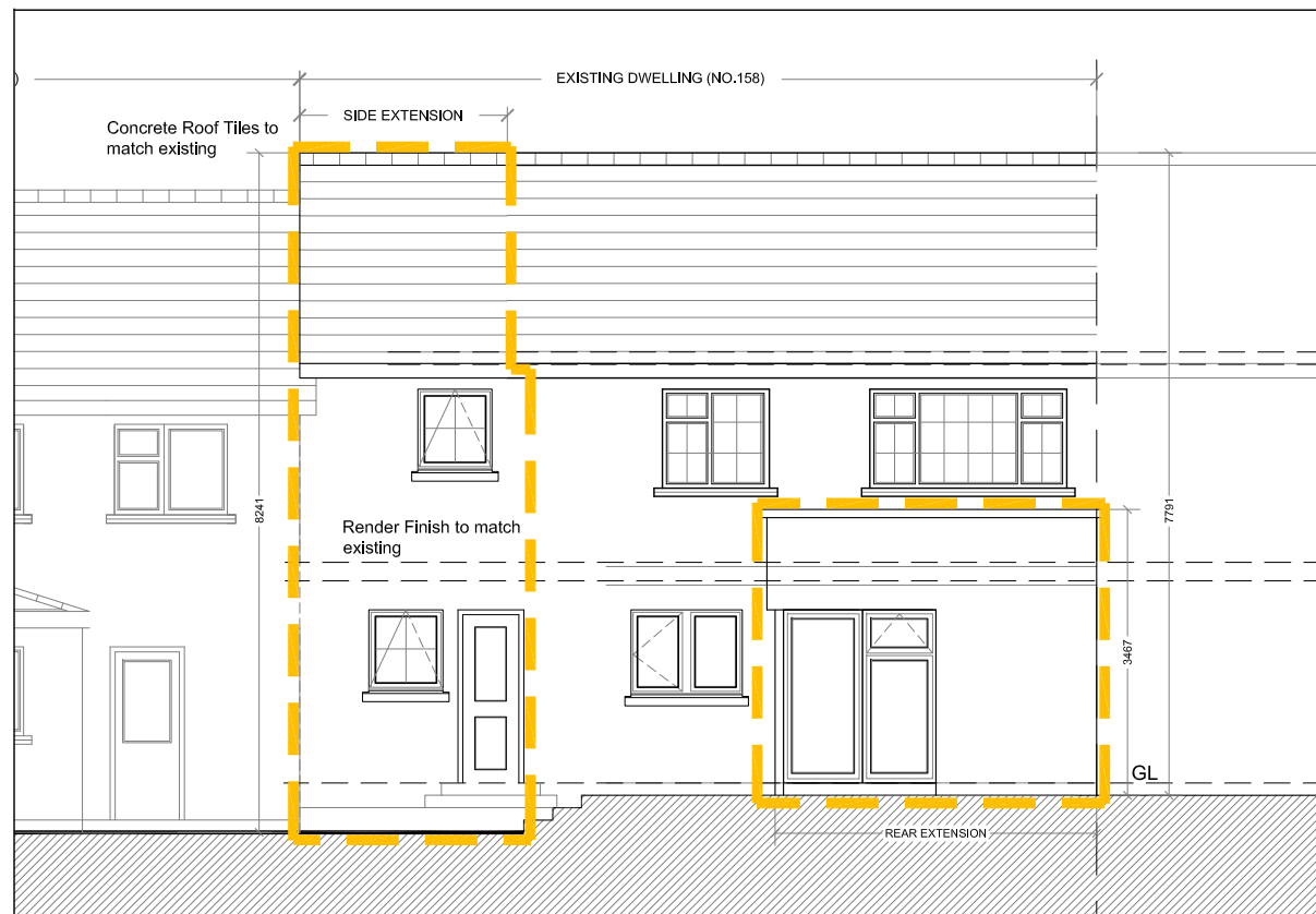
Proposed Rear (North-West) Elevation - Scale 1:100
